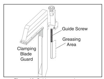
Figure 46. Guide screw greasing area.
